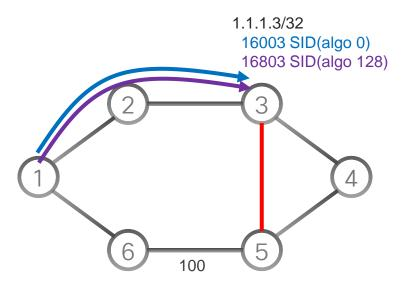
Each node in this topology supports SR alg0, alg128 Default IGP link metric: I:10 At node 1 for destination 3
