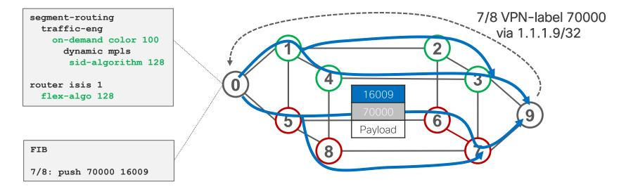
Node 0 automatically steers any BGP route without color from 9 via 16009 (any plane)
